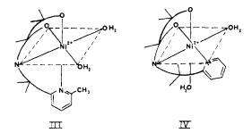
two CH<sub>2</sub> protons. The CH<sub>2</sub> doublet observed for Ni(N-pyr-L-Asp) therefore supports the more strained structure IV for this complex. It should be emphasized, however, that too little is currently known about the origins of such splitting to make unequivocal structural assignments.
